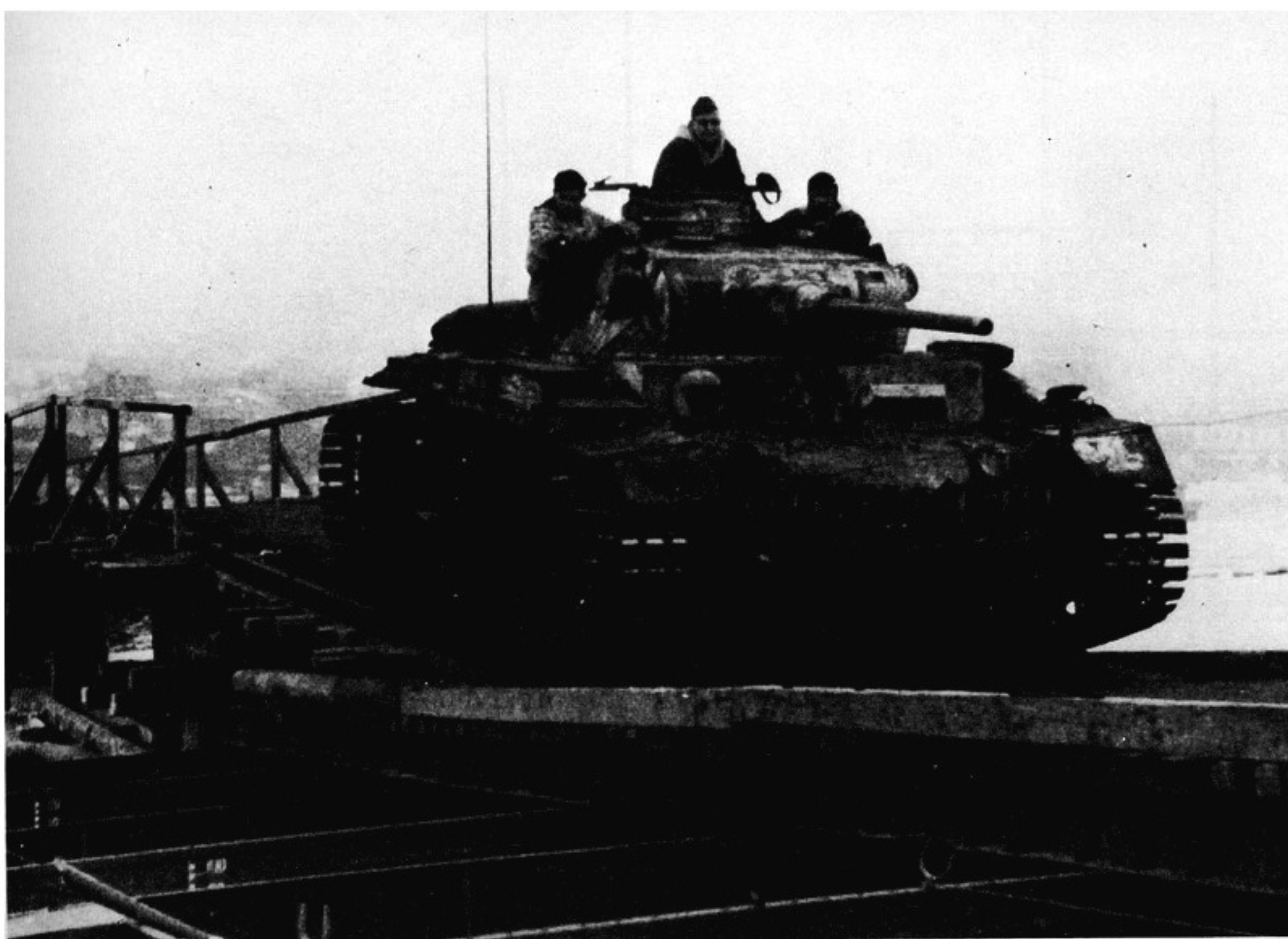
As of 1944, the Panzer III in action on the eastern front were fitted with wider tracks, the so-called "Ostkette." Because of the extra width, the tanks could be driven safely only on flat terrain.
