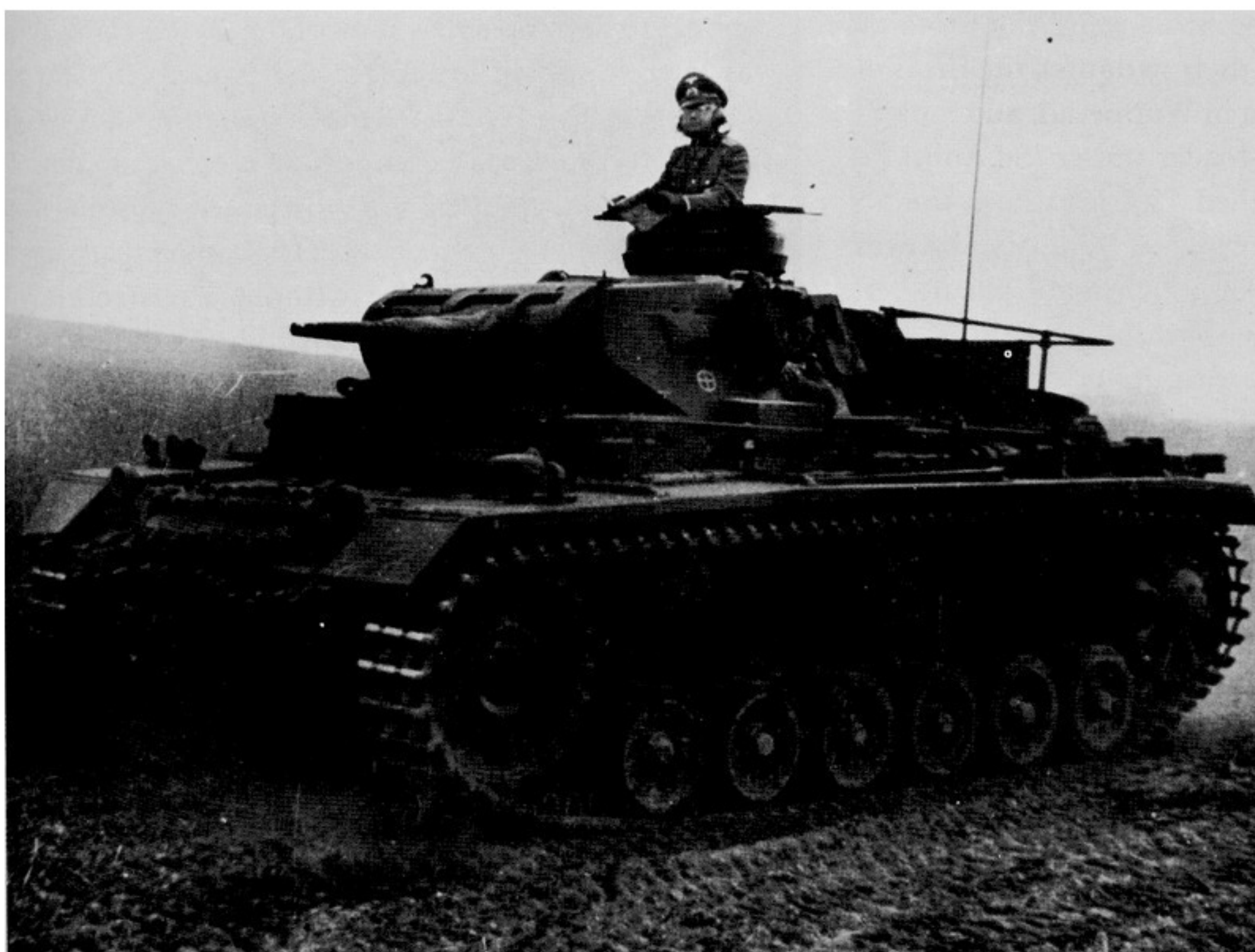
A Command Vehicle III of the 13th Panzer Division in Russia. The picture shows the added antennas. The turret is fixed in position, and the primary weapon is a dummy.
