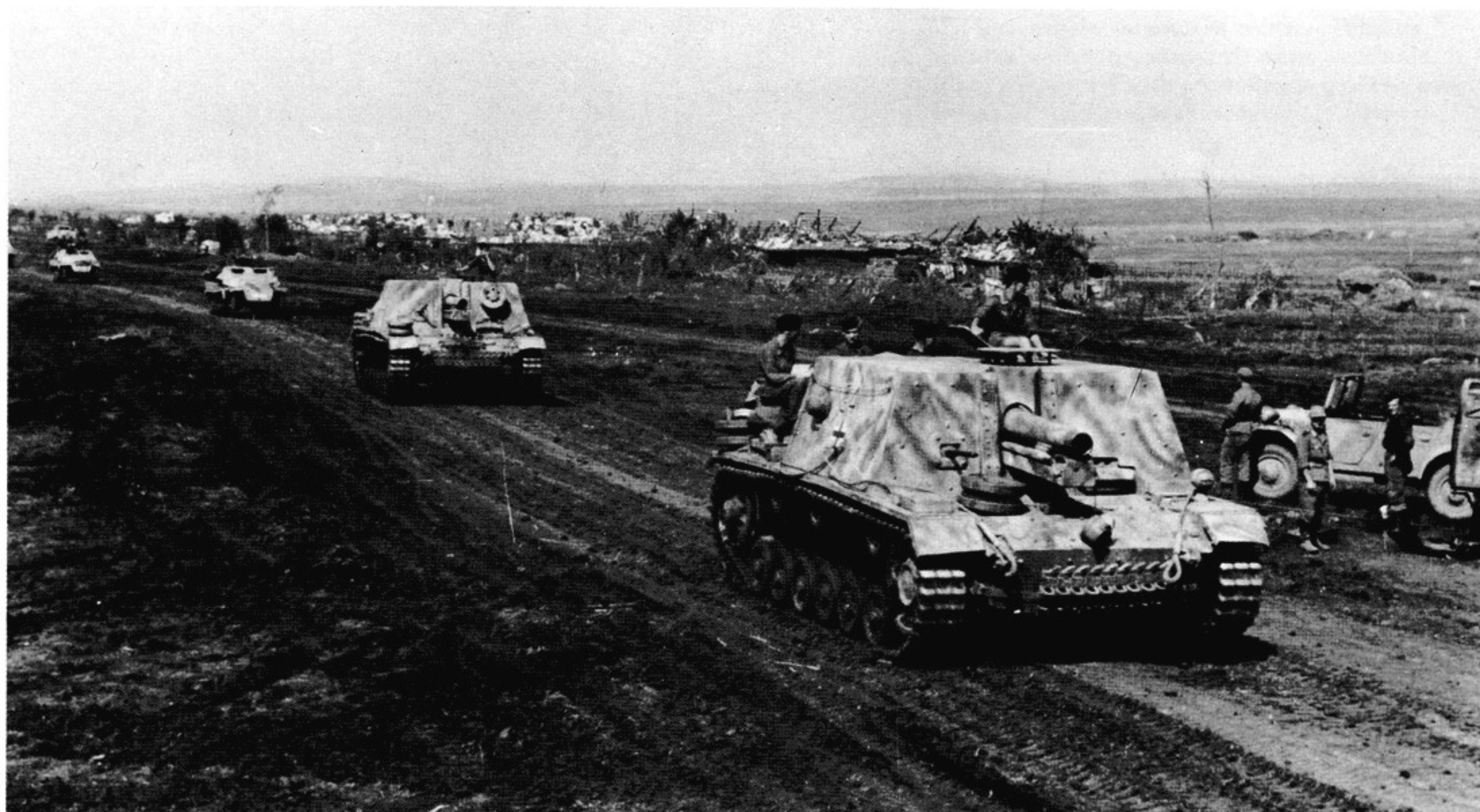
Two more Sturminfanteriegeschütz 33 of Panzer Regiment 201. The picture shows the radio-operator's bow machine gun, used for close combat. Next to the first vehicle is a light "standard" passenger vehicle.
