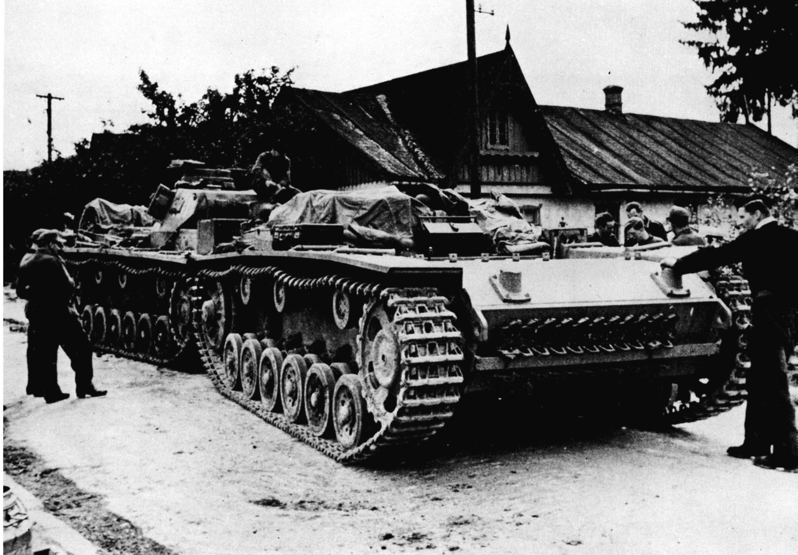
Most of the mustered-out Panzer III chassis, though, were used for tank recovery vehicles. They provided valuable service in towing broken-down armored vehicles. A large percentage of these vehicles came into being when the troops rebuilt them.
