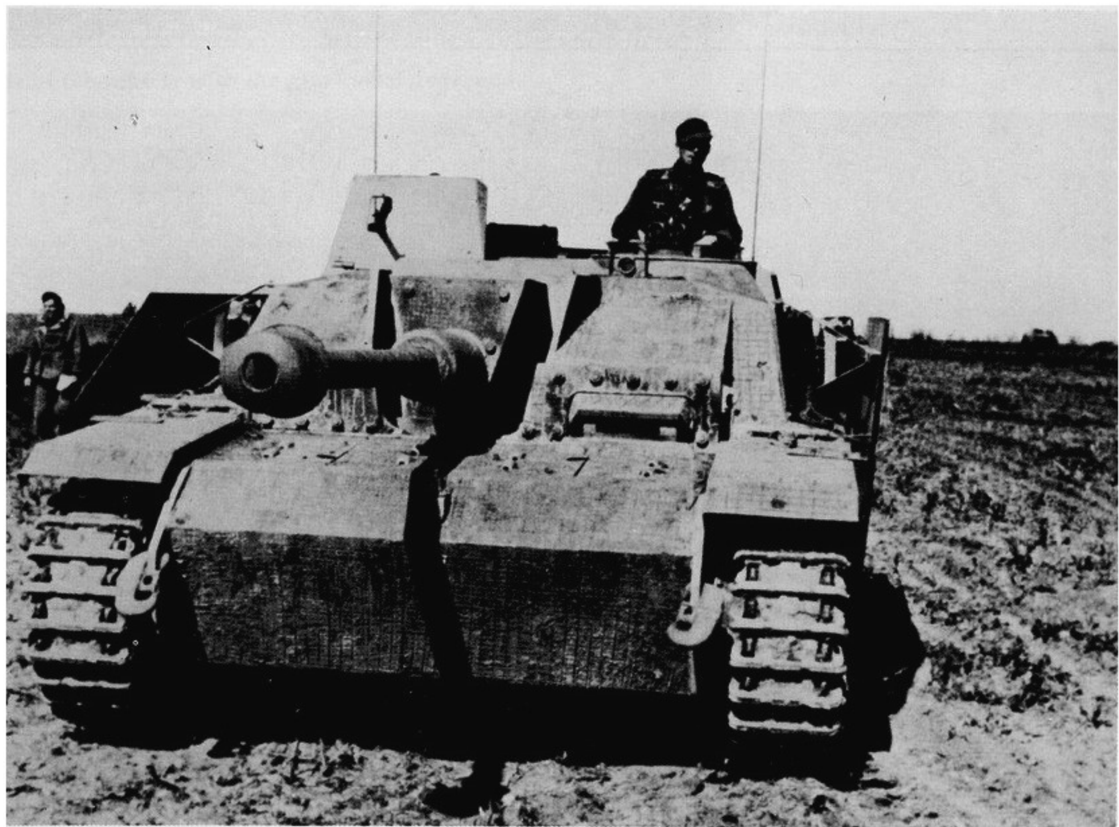
The Ausf. G version of the Sturmgeschütz 40 appeared in 1943 and had a wider superstructure. The gun commander now had a commander's cupola at his disposal.
