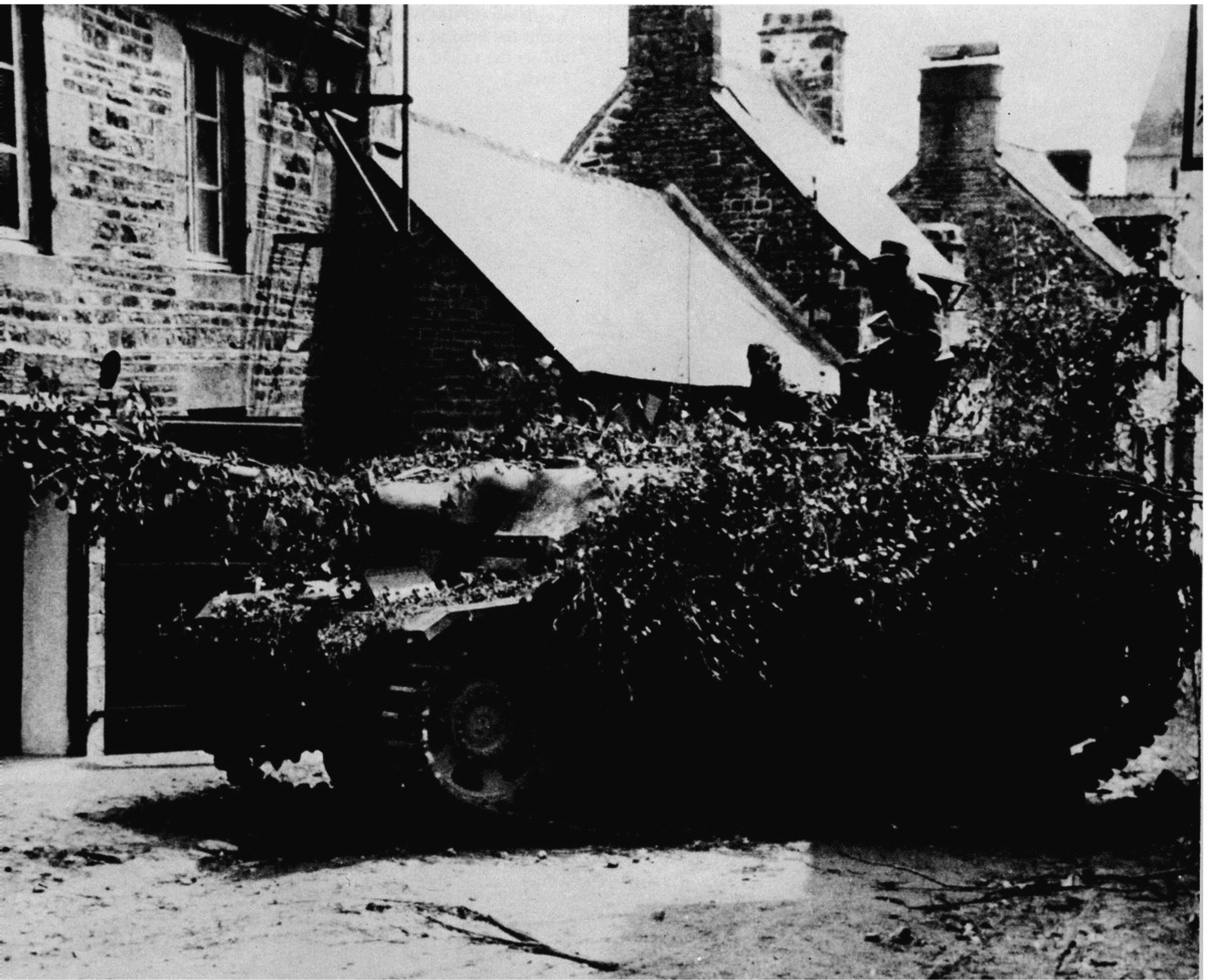
A camouflaged Sturmgeschütz in action on the western front. The picture shows a modified type of apron attachment. The concrete shot deflector in front of the cupola can also be seen.
