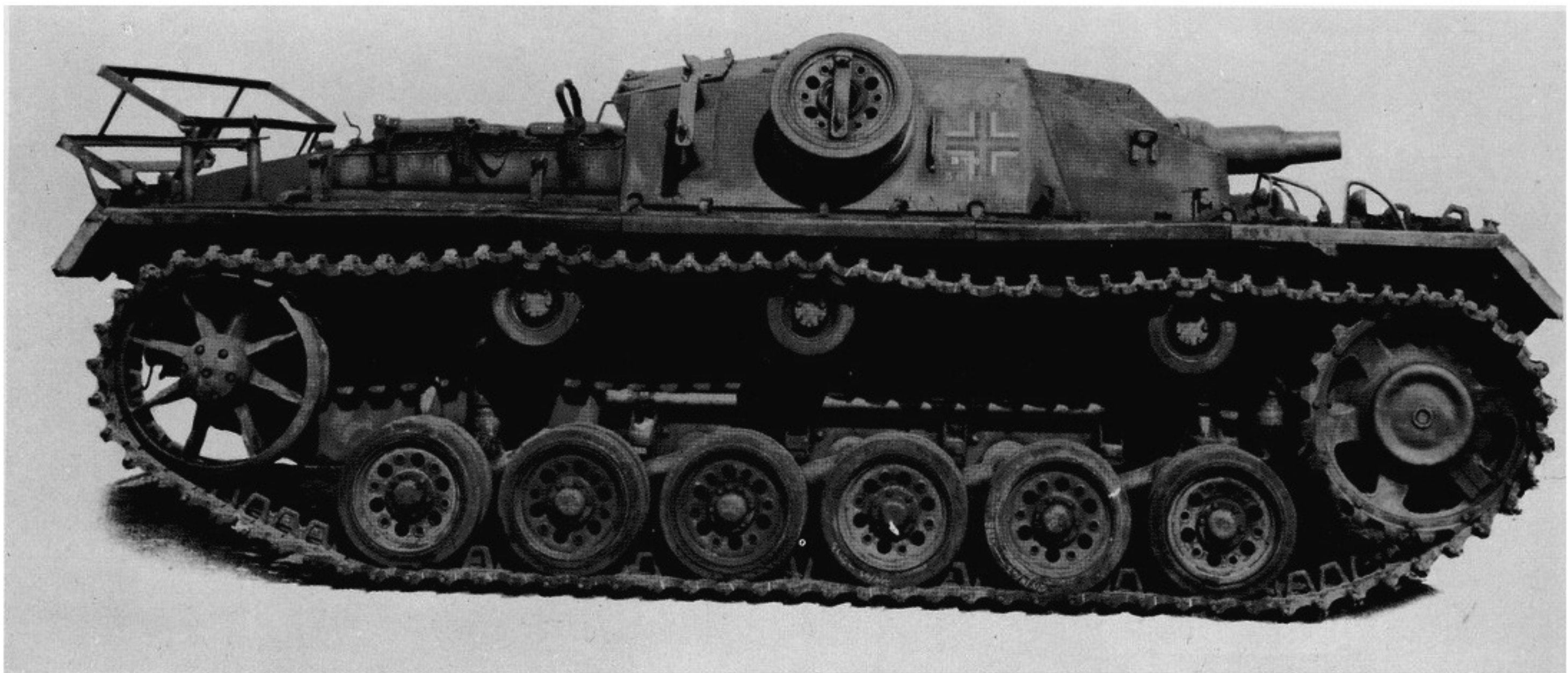
This side view of Sturmgeschütz shows the low superstructure of the vehicle as well as the short 75mm Sturmkanone. Spare torsion bars were sometimes stored on the sides of the hull above the road wheels.
