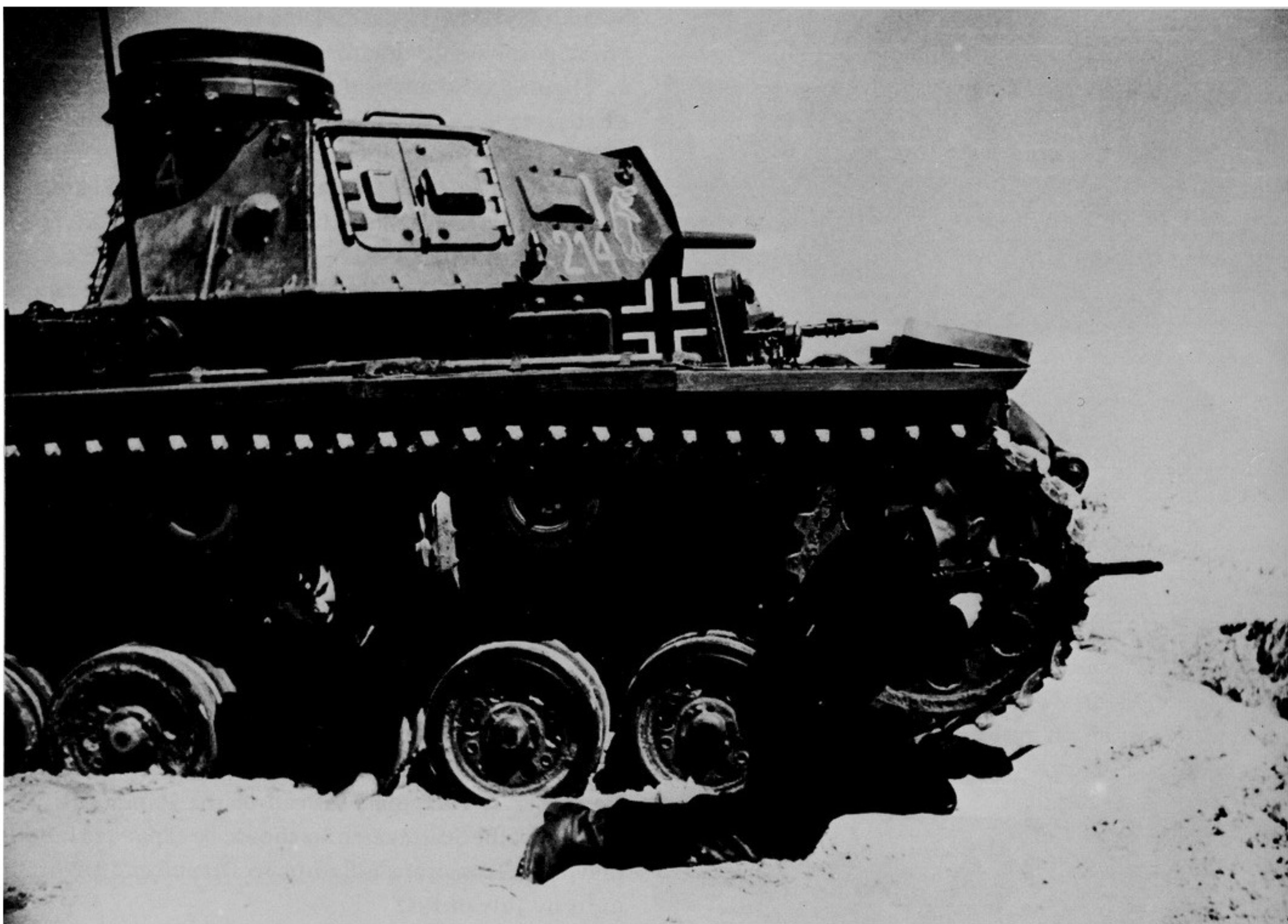
The crew practices leaving and Ausf. G tank modified for submerging. The two machine guns could be removed quite easily for use in close-range defense outside the vehicle.
