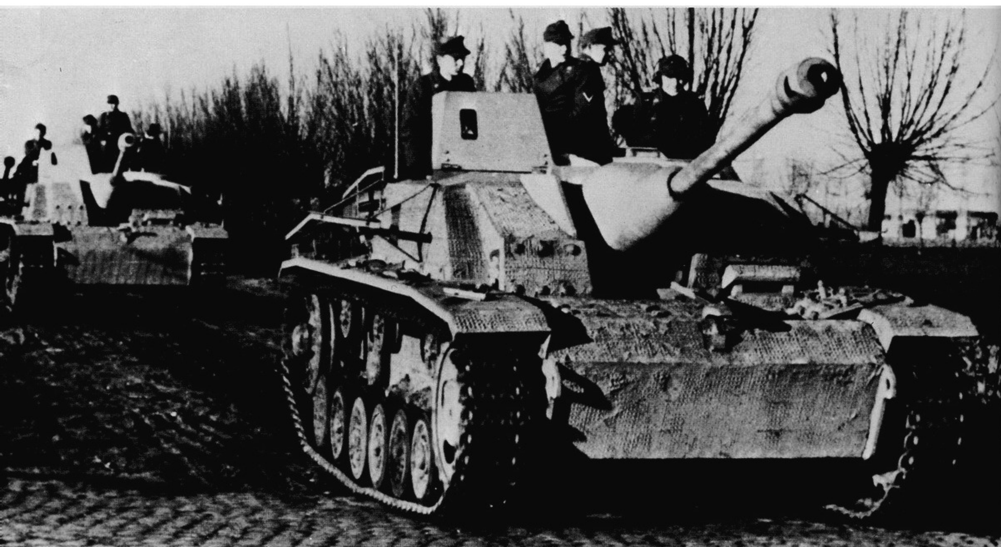
The angular gun-mantle armor was a typical identifying mark of all assault-gun versions for some time. As of mid-1943 it was partly replaced by a cast steel fitting in shot-deflecting form, the so-called "Saukopf."
