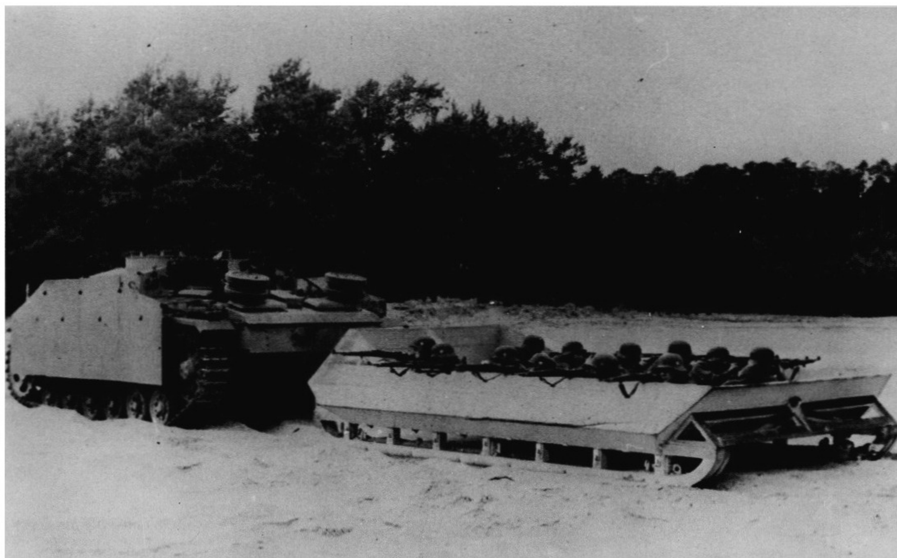
Crew sleds in the Russian manner were tested as a means of waging mobile winter warfare. This picture shows such a sled hitched to a Sturmgeschütz 40 Ausf. G.
