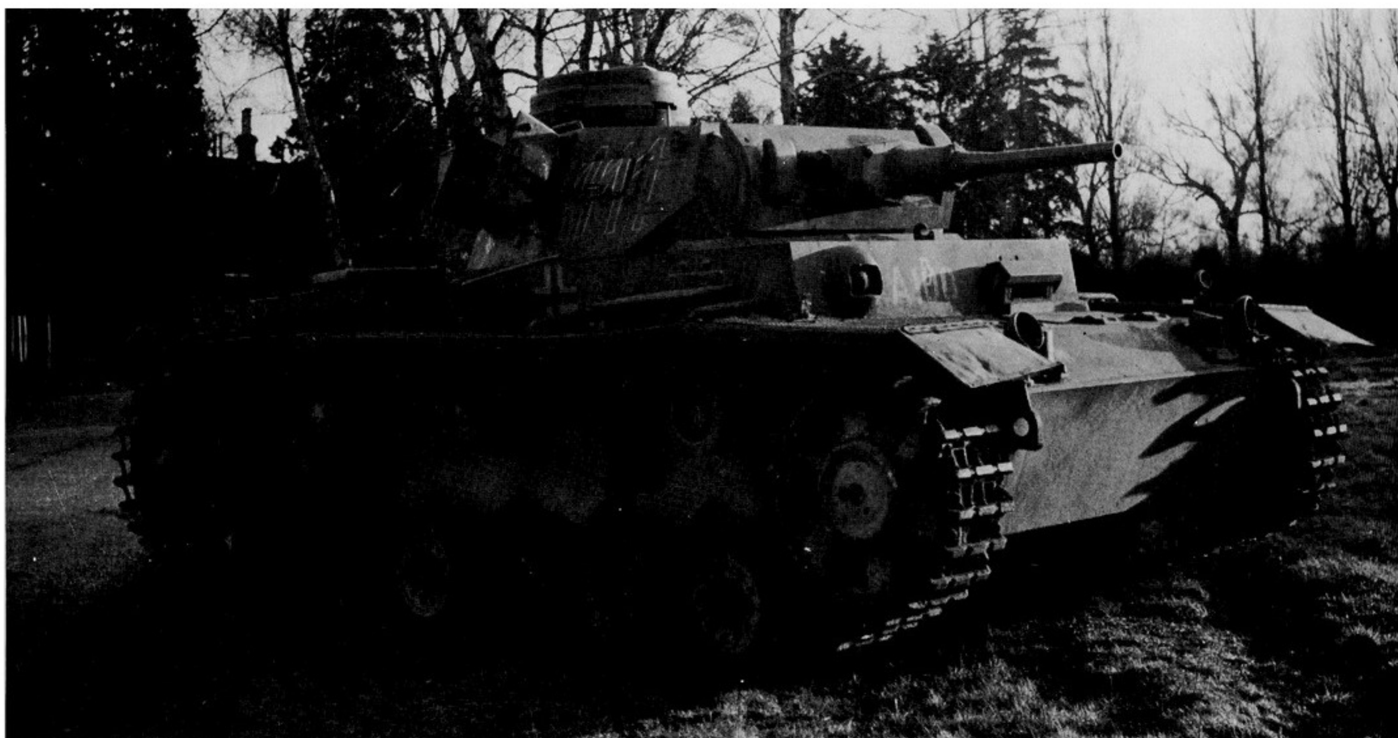
The first series of Ausf. J was still fitted with the short 50mm KwK L/42 gun.
