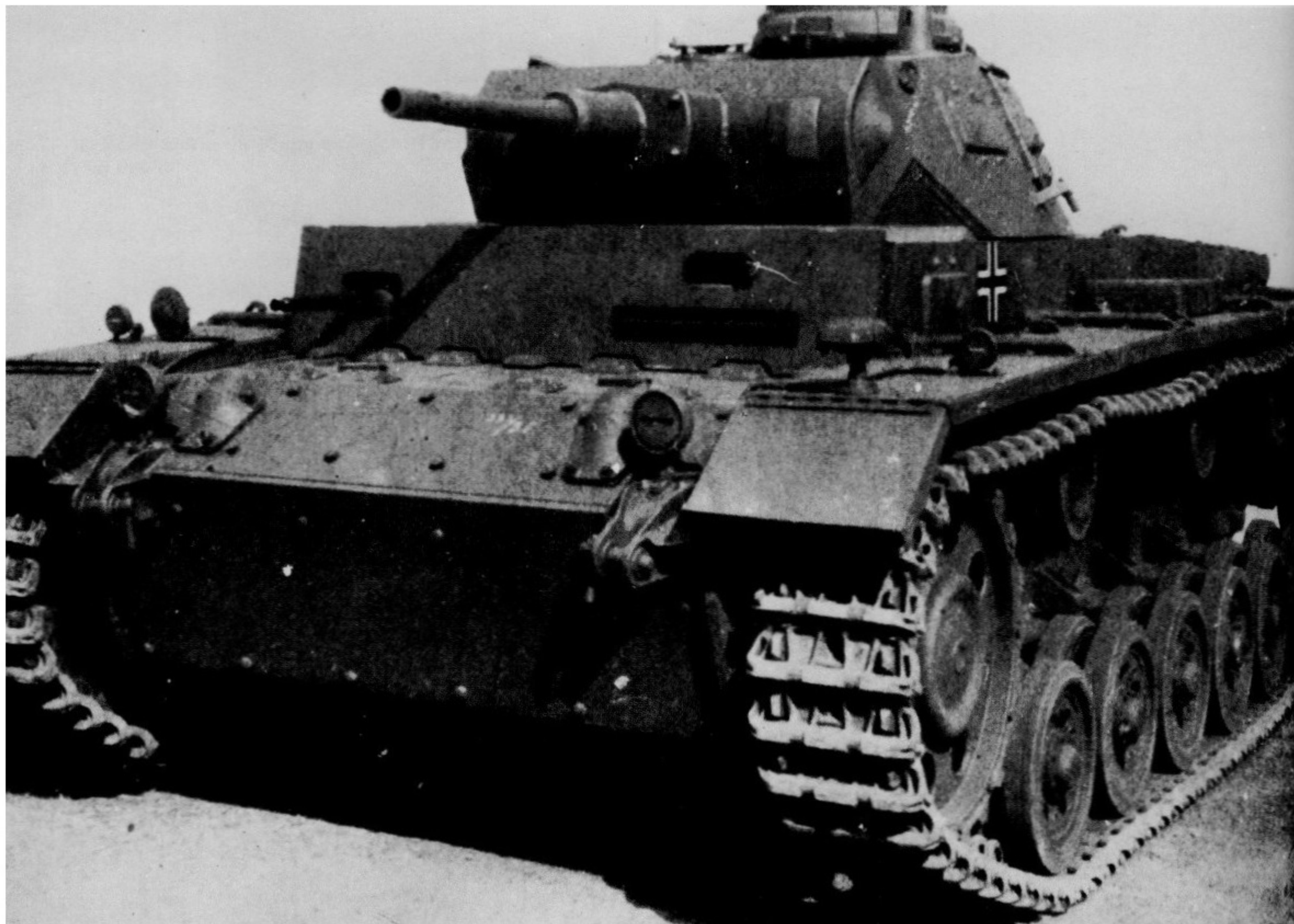
This picture shows a Panzer III Ausf. E or F which was later rearmed with the 50mm KwK L/42. The front armor of the Ausf. E to H was later strengthened by screwed-on or welded-on 30 mm armor plate.
