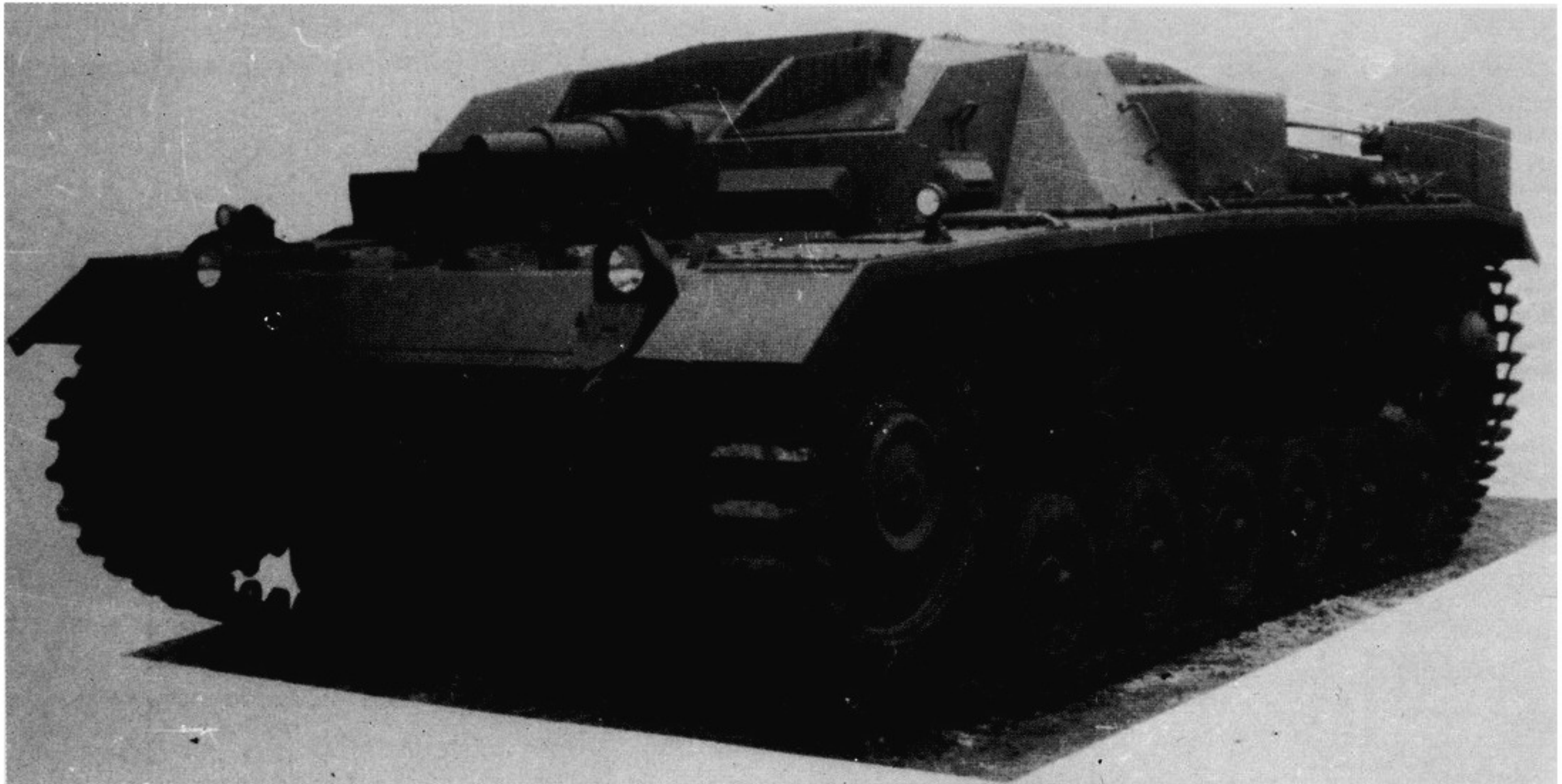
The round assembly ports in the bow plate had been eliminated from Ausf. A. The open sight tunnel was retained.
