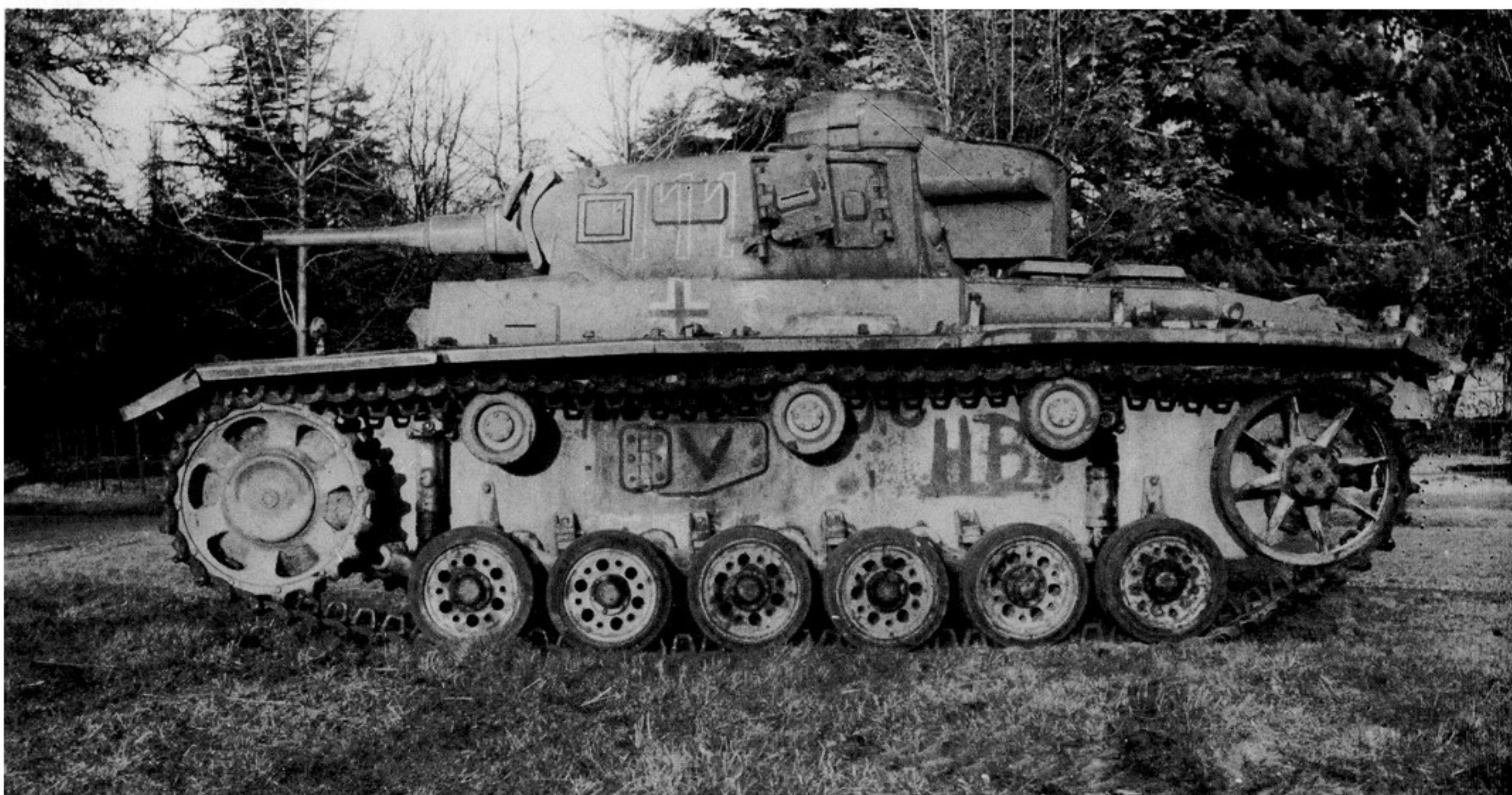
The first series of Ausf. J was still fitted with the short 50mm KwK L/42 gun.
