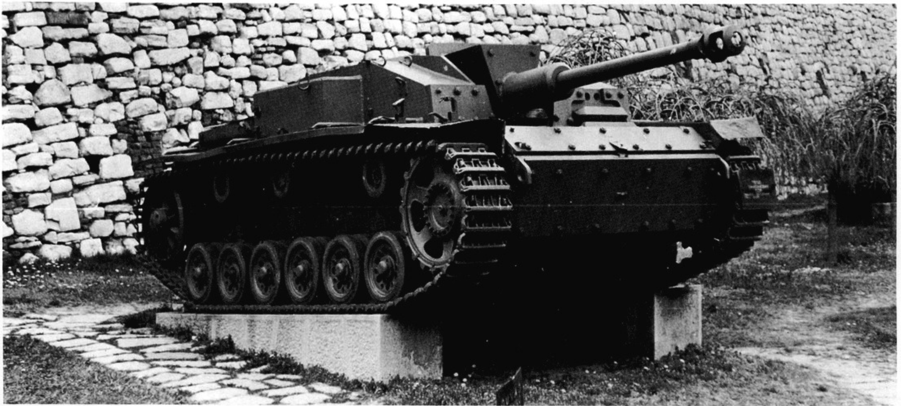
An L/48 gun with additional 30 mm armor plate on the front. This picture shows such a Ausf. F/8 vehicle.
