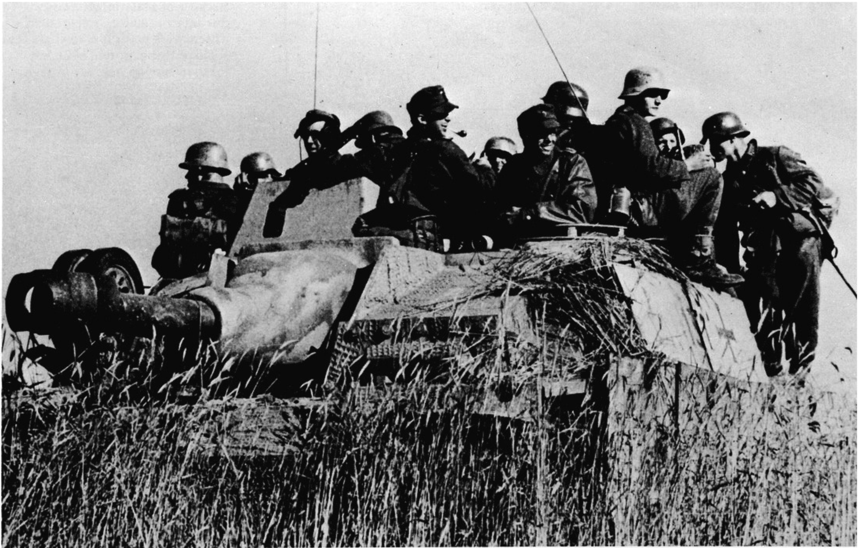
A "Saukopf" ("pig's-head") mount was also introduced for the 105mm Sturmhaubitze, but it was actually installed in only some vehicles. This picture shows such a vehicle with the new mount and muzzle brake.
