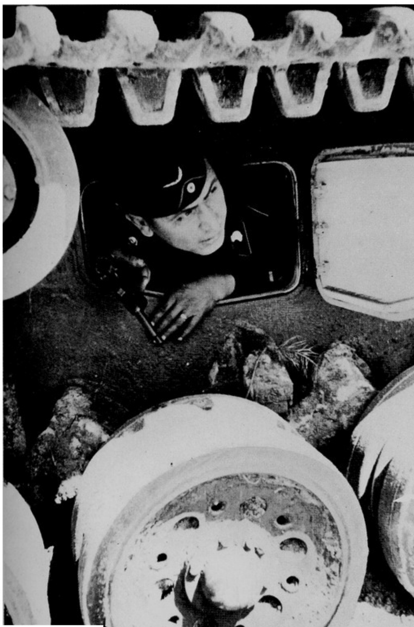
During production of the Ausf. L, the emergency exit hatches located in both sides of the hull since Type E were eliminated.
