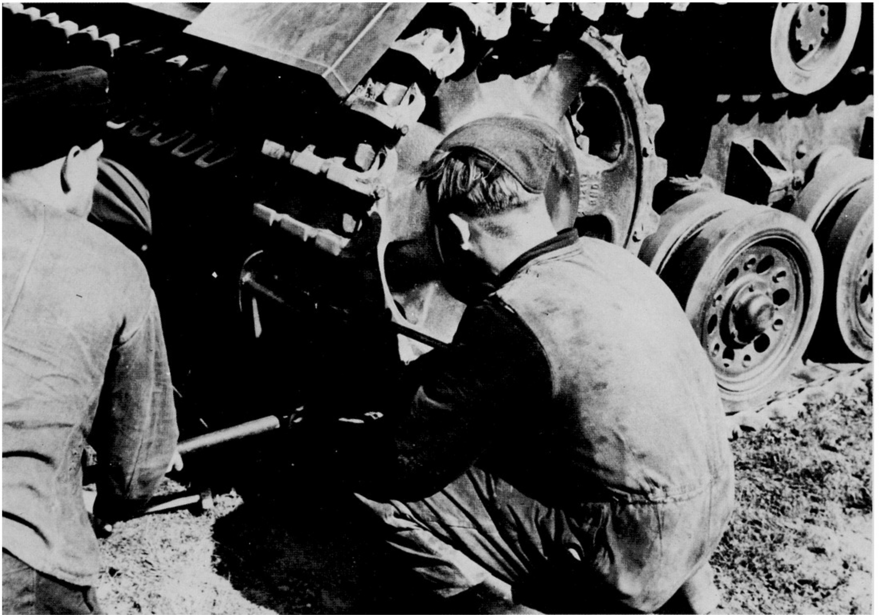
The most vulnerable parts of any tank are its tracks. Changing track links was practiced frequently to assure the readiness of the vehicles. This picture shows the use of special tools to reconnect the track.
