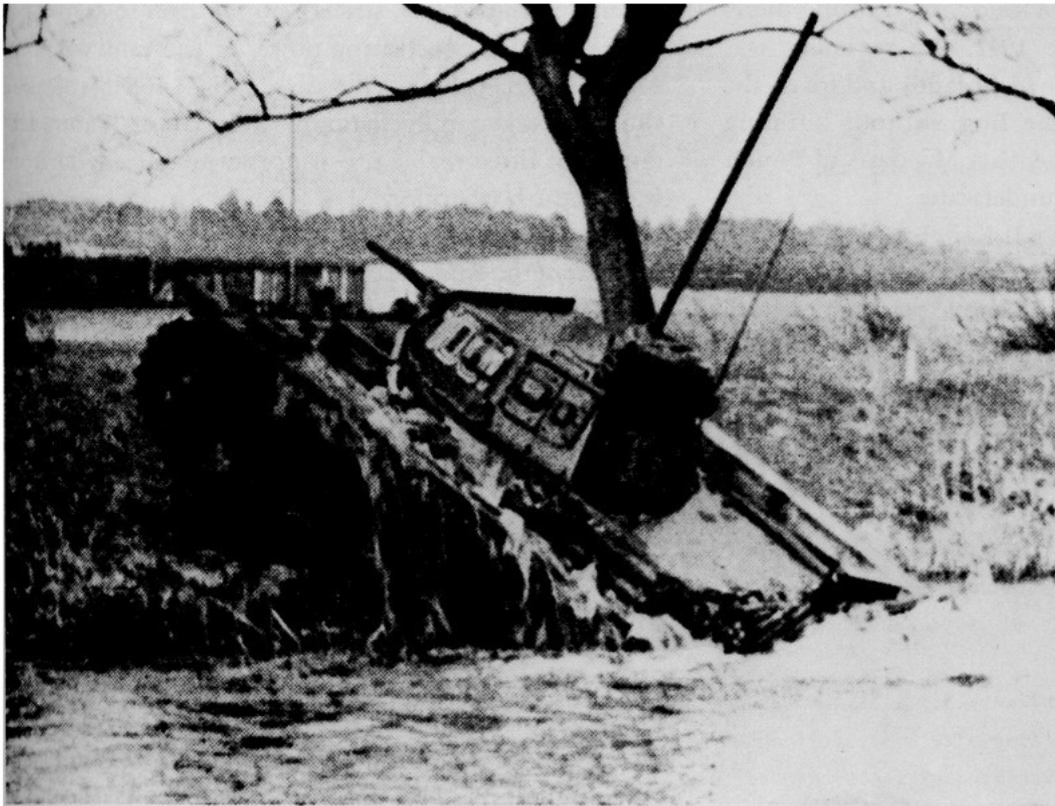
After "Operation Sealion" was given up, some of the diving tanks were turned over to the 18th Panzer Division. At the beginning of the Russian campaign in 1941, they crossed the Bug underwater. Instead of an air-supply hose, the vehicles used a steel pipe 3.5 meters long.
