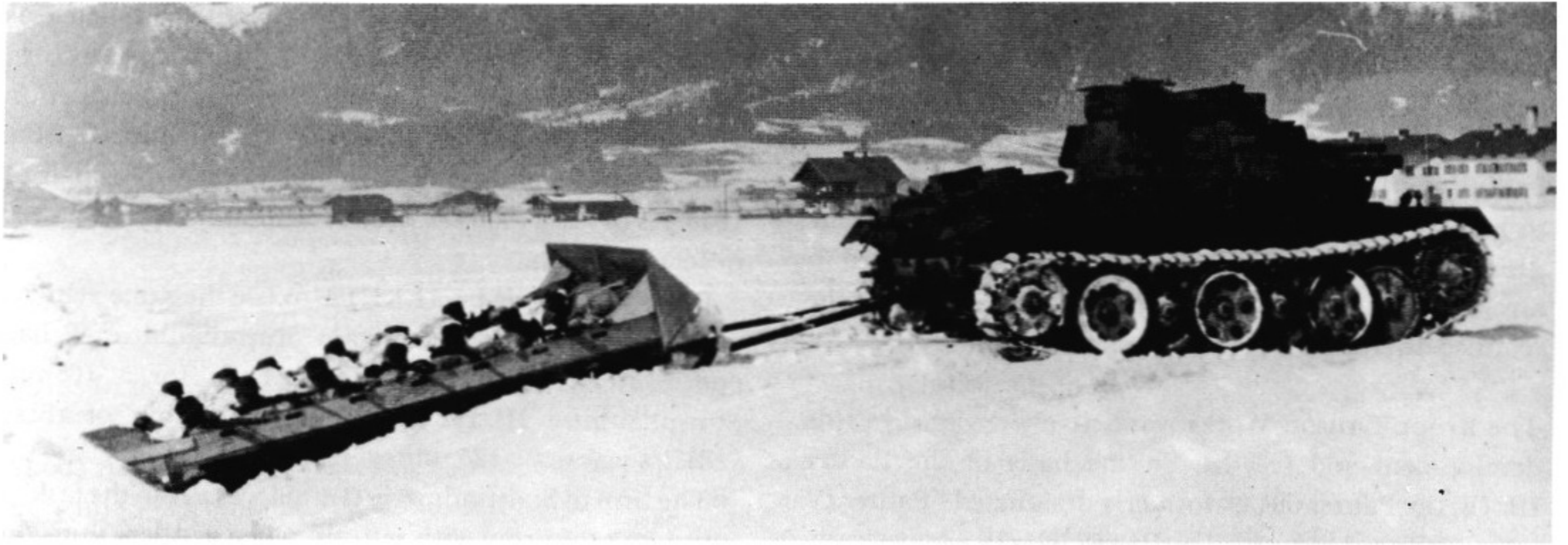
After thorough winter testing, these vehicles were also used to pull the heavy sled trailers made for tracked vehicles.
